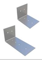
Clark Dietrich aluminum burn clips are used as part of the H-stud area separation wall assembly and are designed to melt when exposed to fire. The clips hold the area separation wall assemblies in place at the floor, roof and truss line between adjacent units. In a fire, the aluminum burn clips on the fire-ridden side of the wall will melt, allowing the wall structure for that side to collapse.
